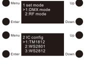
1. Set mode: to select an operation mode, click "Enter" button to enter the configuration interface, then click "Up" and "Down" buttons to choose RF or DMX mode, click "Menu" button to confirm the setting and return to menu selection interface.
