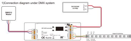
Note: Each terminal can support 10A rated current, Please note that when connecting the light strips, do not exceed this load.
